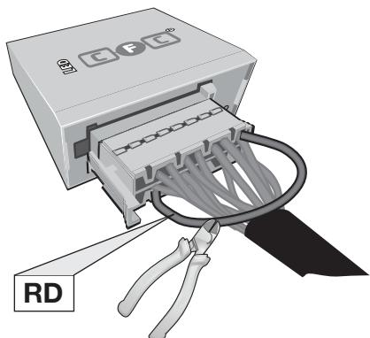
Pin 11 and Pin 2 disconnected
